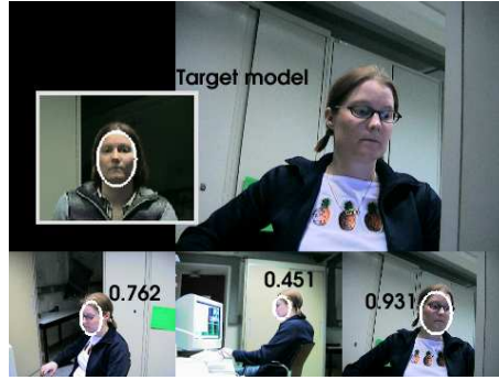
Fig. 3. The best view selection according to the Bhattacharyya coefficients of the individual trackers is shown. The small images at the bottom show the tracking results of the individual camera trackers as white ellipses. The numbers represent the corresponding Bhattacharyya coefficients. In the top row the used target model and the output of the virtual editor are displayed.
