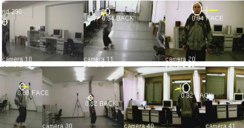
Figure 7: Color histograms of detected heads are compared to the target histograms and a “face/back” decision is made. The view with the most confident face decision is selected.
