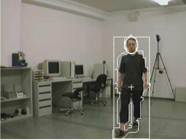
Figure 2: Each incoming image is processed to find connected components in a segmented image to determine the silhouettes around them and to detect heads (white ellipse) at the top of the silhouettes. The rectangle is a bounding box around the segmented component.
