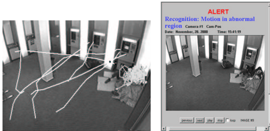
Figure 8. Detection of an unusual motion event caused by the two unauthorized people which improperly occupy the bank lobby using it as a dormitory. In the left image, the current situation of the surveillance framework is illustrated while in the right image the alert seen by the security staff is shown.
