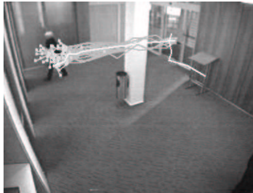
Figure 6. The development of a new prototype curve caused by the person crossing the bank lobby is illustrated in white.
