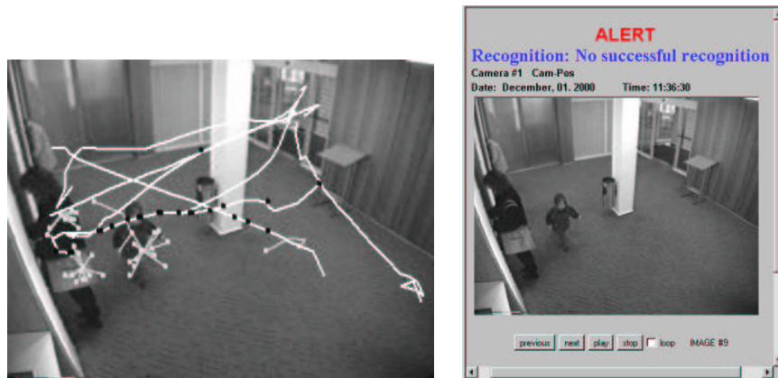
Figure 10. Detection of an unusual motion event caused by the child running around the pillar.
